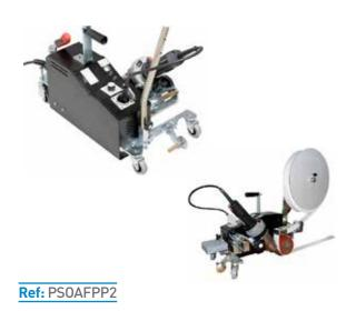
The automatic welding machine FORPLASTP2 is an efficient and manoeuvrable device for welding truck tarpaulins, tents, awning materials and advertising banners.
